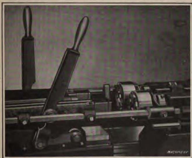
Fig. 5. Threading Machine provided with Special Blank-holders
